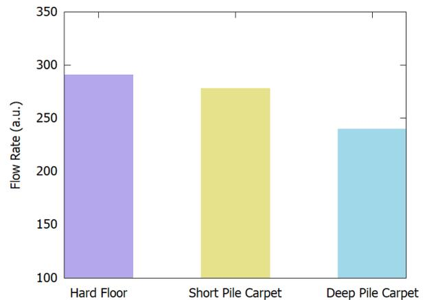
With constant power draw, there can be up to a 20% drop in mass flow rate on thicker carpets.
